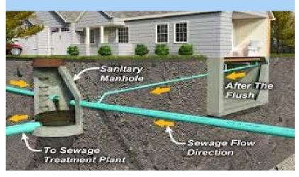
Wastewater flows from house into closed gravity piping system and is pumped to WWTP for treatment.
