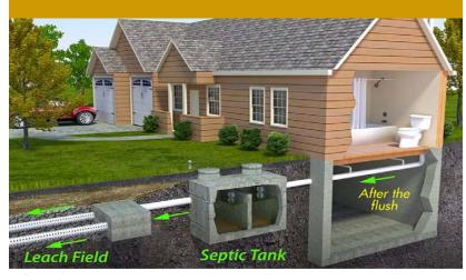
Wastewater flows from house through septic tank and drain field into the soil and groundwater and surface water.
